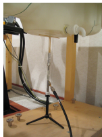
Photo of the dipole Antenna
