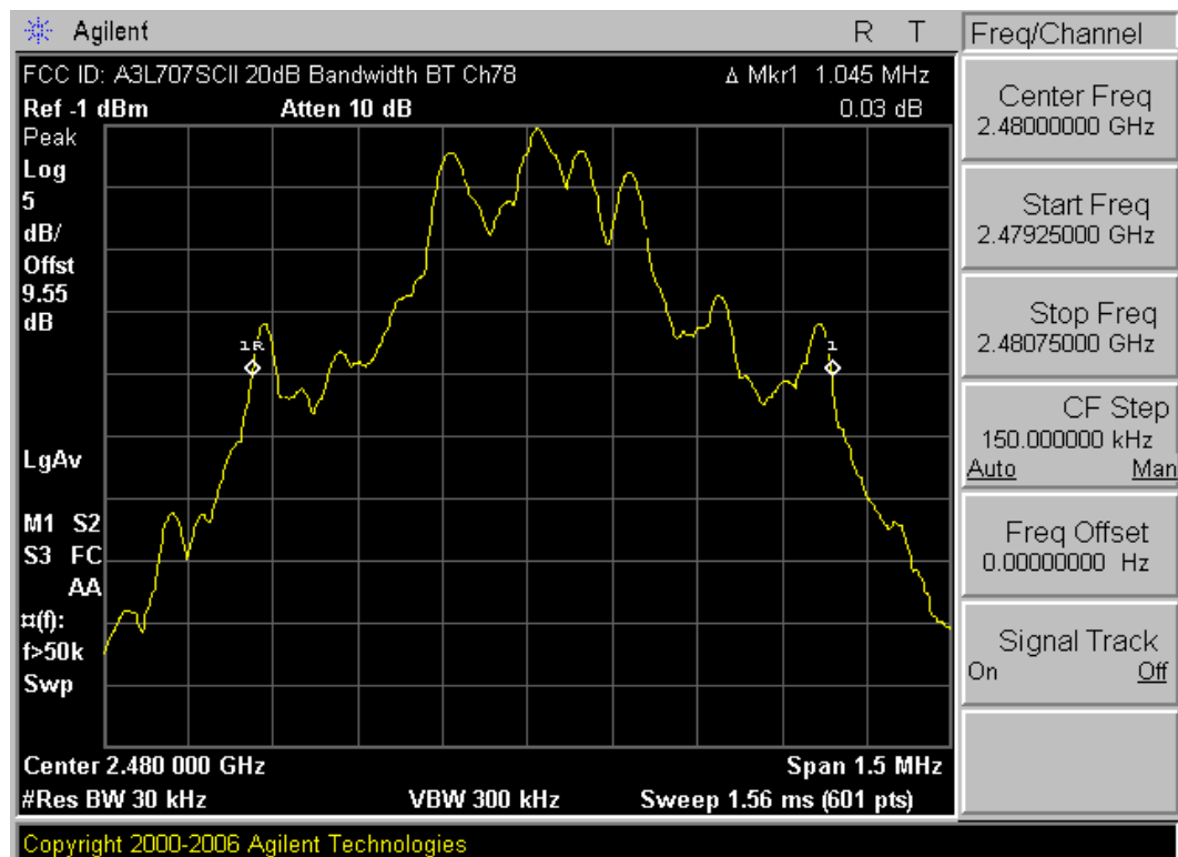
Plot 6-3. 20dB Bandwidth Plot (Bluetooth – Ch. 78)
