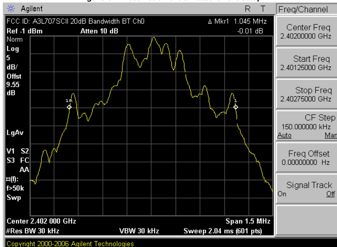
Plot 6-1. 20dB Bandwidth Plot (Bluetooth – Ch. 0)
