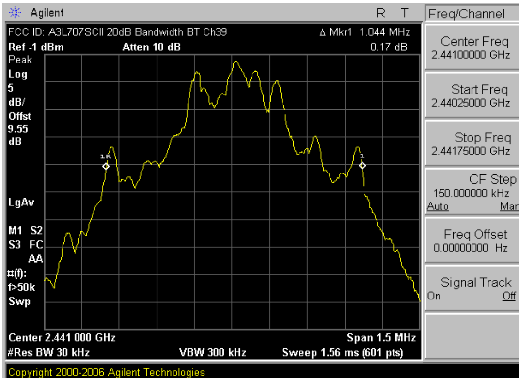
Plot 6-2. 20dB Bandwidth Plot (Bluetooth – Ch. 39)
