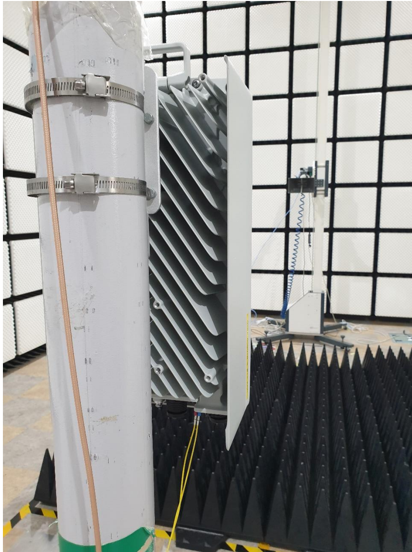
Radiated Test Setup Photo – Spurious (1 GHz ~ 18 GHz, H)
