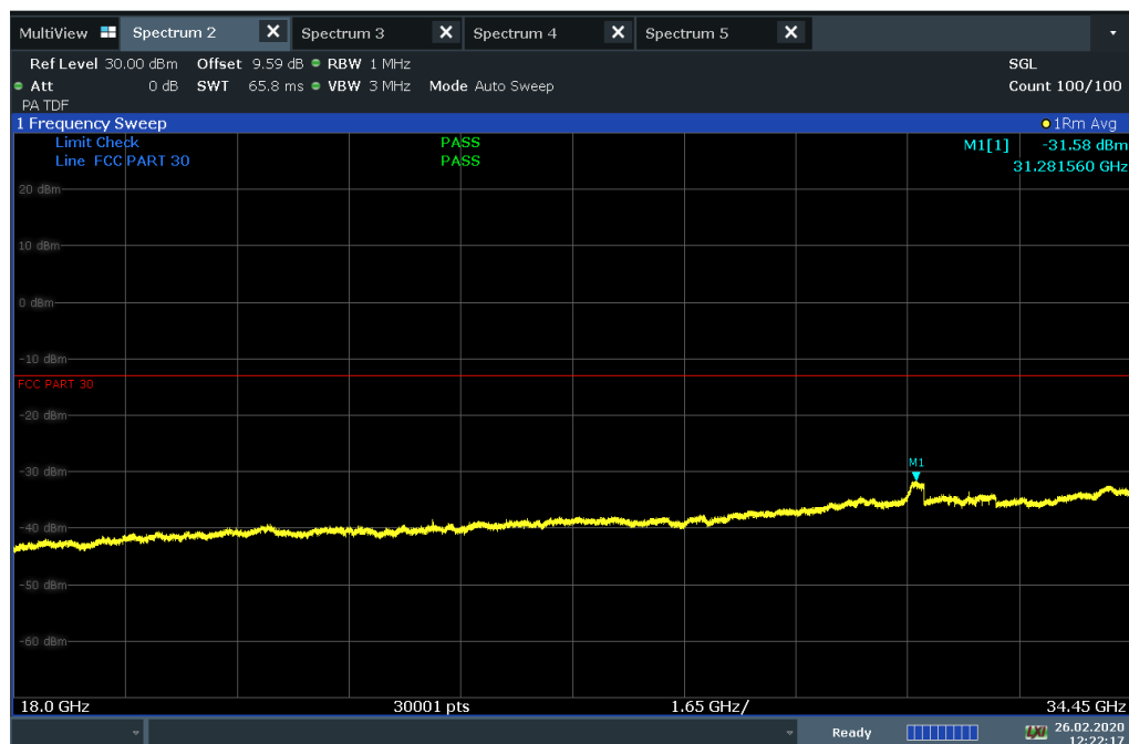
Plot 7-308. Radiated Spurious Plot 18-33 GHz (8CC QPSK Low Ch. Ant. Angle 45, Final)
