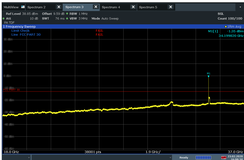
Plot 7-344. Radiated Spurious Plot 18-37 GHz (1CC QPSK High Ch. Ant. Angle 135, Final)
