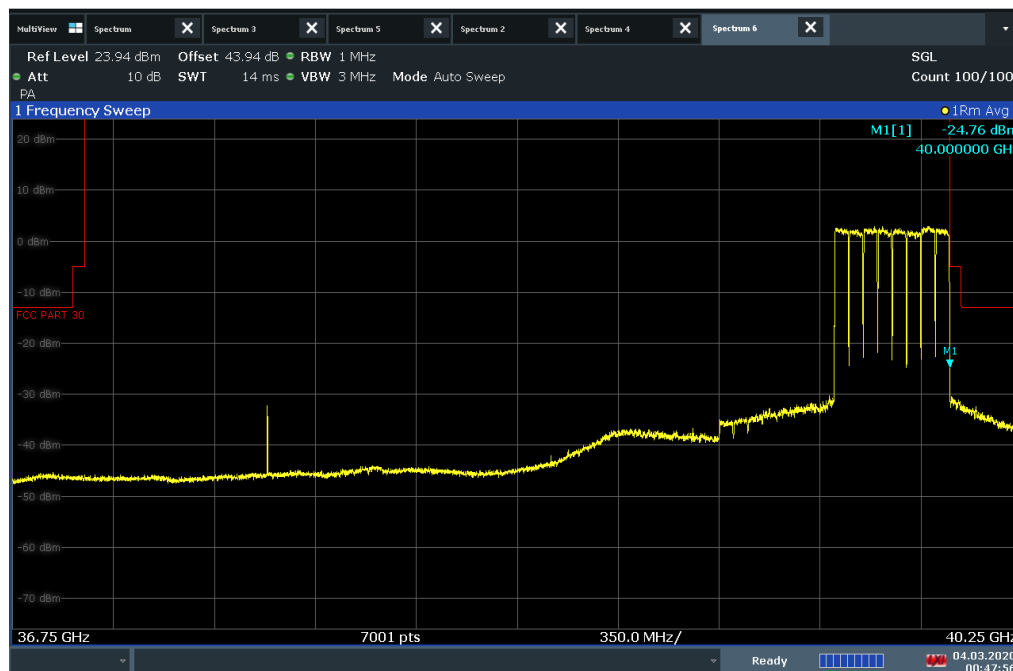
Plot 7-521. Band Edge Plot (50MHz BW 8CC QPSK High Channel)
