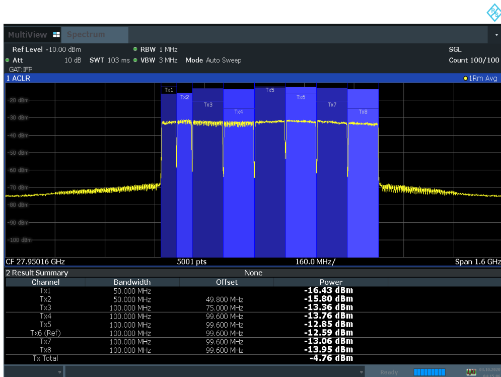
Plot 7-156. EIRP Density (Ant B 50 MHz 2CC + 100 MHz BW 6CC QPSK High)
