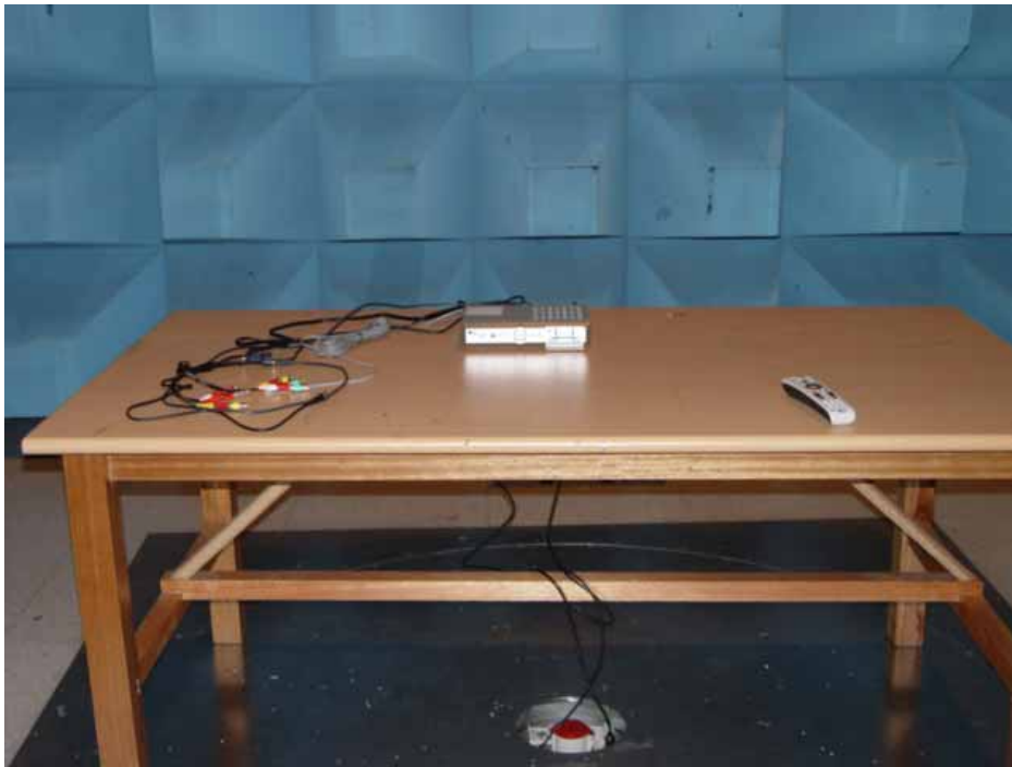
Picture 2. Radiated Emission (Front)
