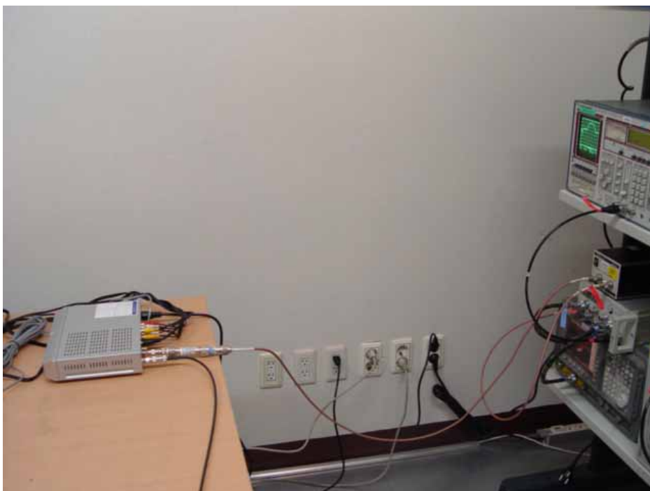
Picture 5. Output Terminal Conducted Spurious Emission
