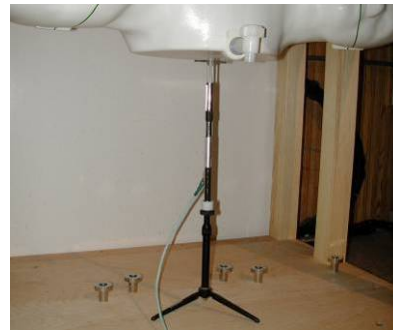
Figure 9-2 System Verification Setup Photo
