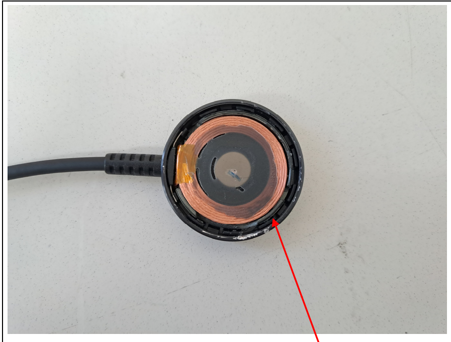
Loop coil antenna
