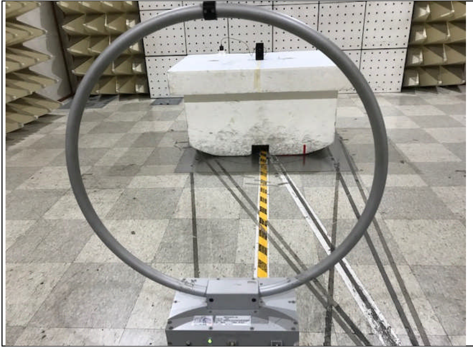
Photo of Test Set up (9 kHz ~ 30 MHz)
