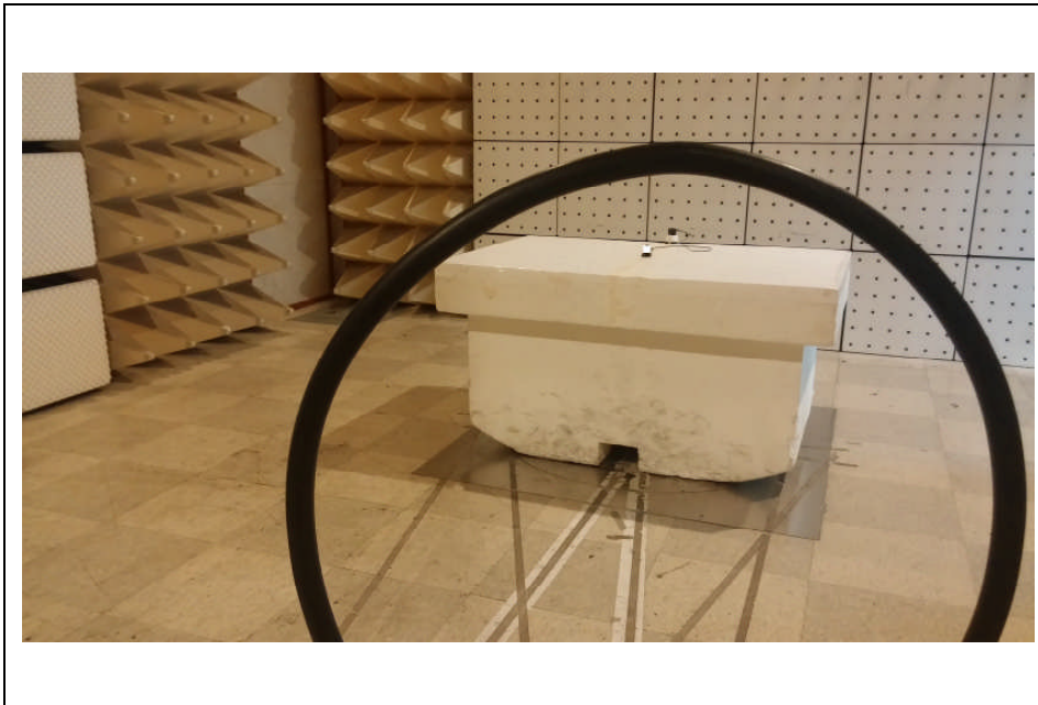
Photo of Test Set up for RSE (9 kHz ~ 30 MHz)
