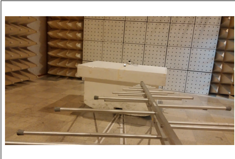
Photo of Test Set up for RSE (30 MHz ~ 1 GHz)
