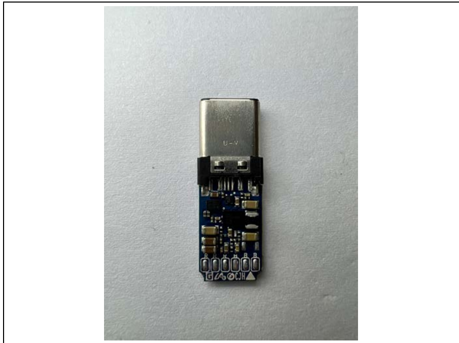
Bottom view of Main PCB
