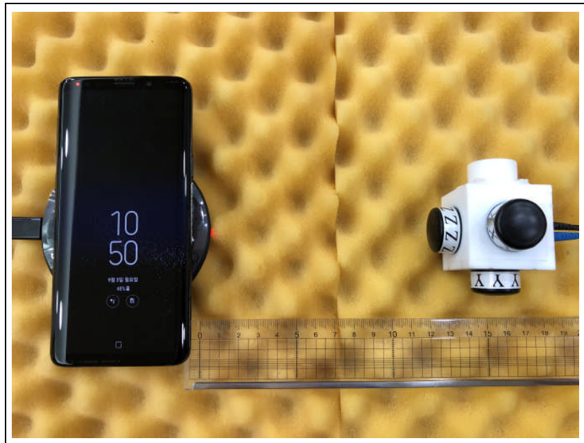
Photo of MPE Test Set up (E-field)
