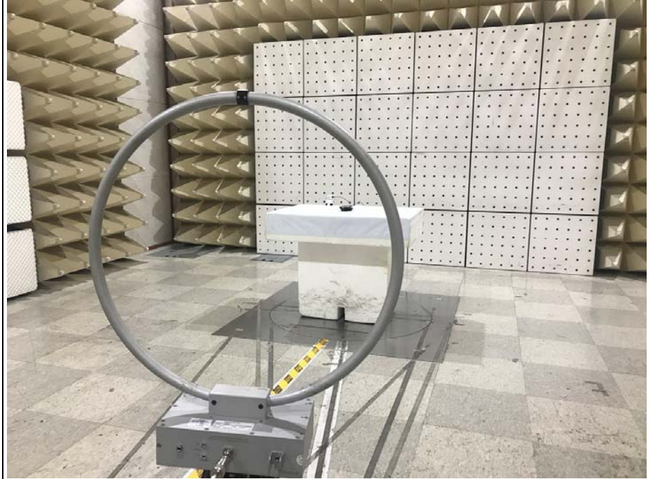
Photo of Test Set up (9 kHz ~ 30 MHz)
