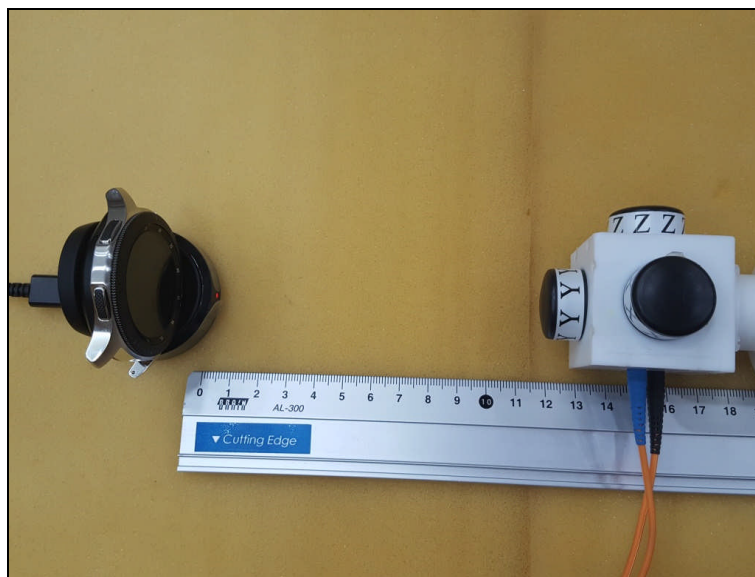
Photo of MPE Test Set up (E-field)
