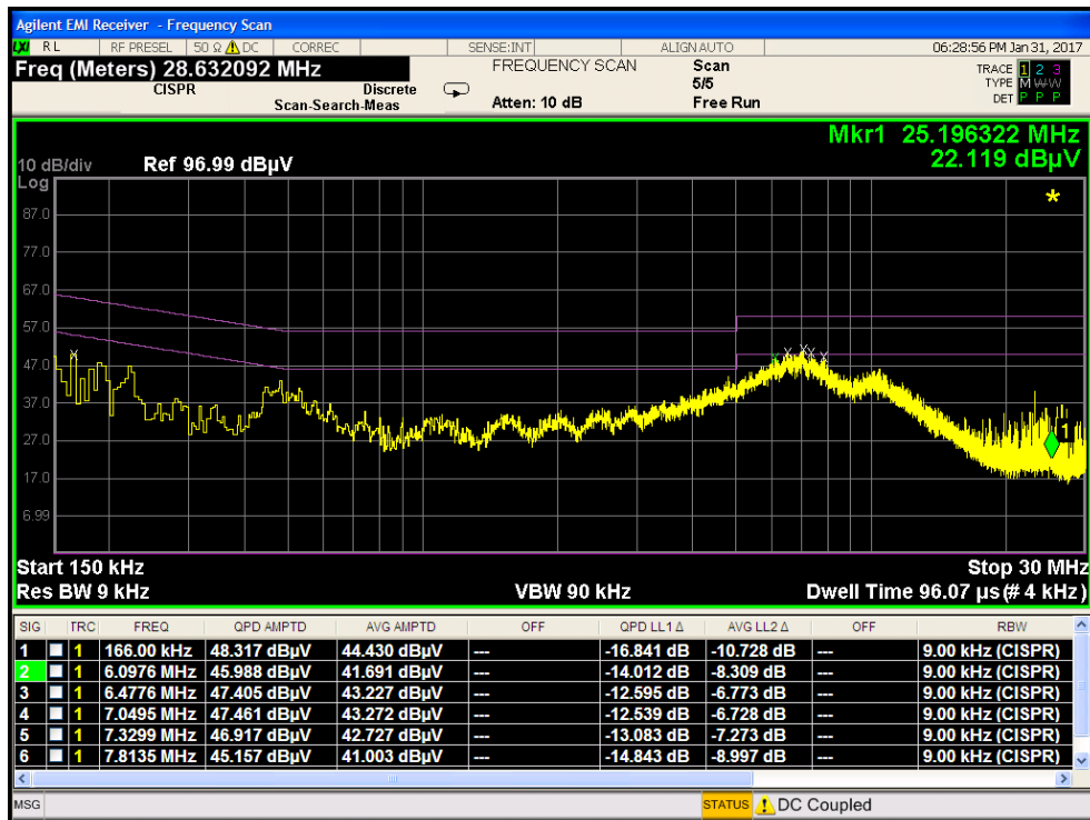
Plot 7-249. Line Conducted Plot with 802.11a UNII Band 3 (L1)
