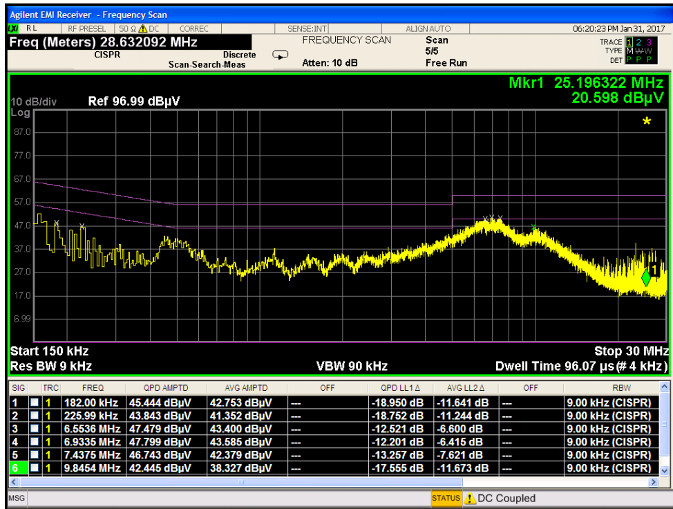
Plot 7-259. Line Conducted Plot with 802.11a UNII Band 1 (L1)
