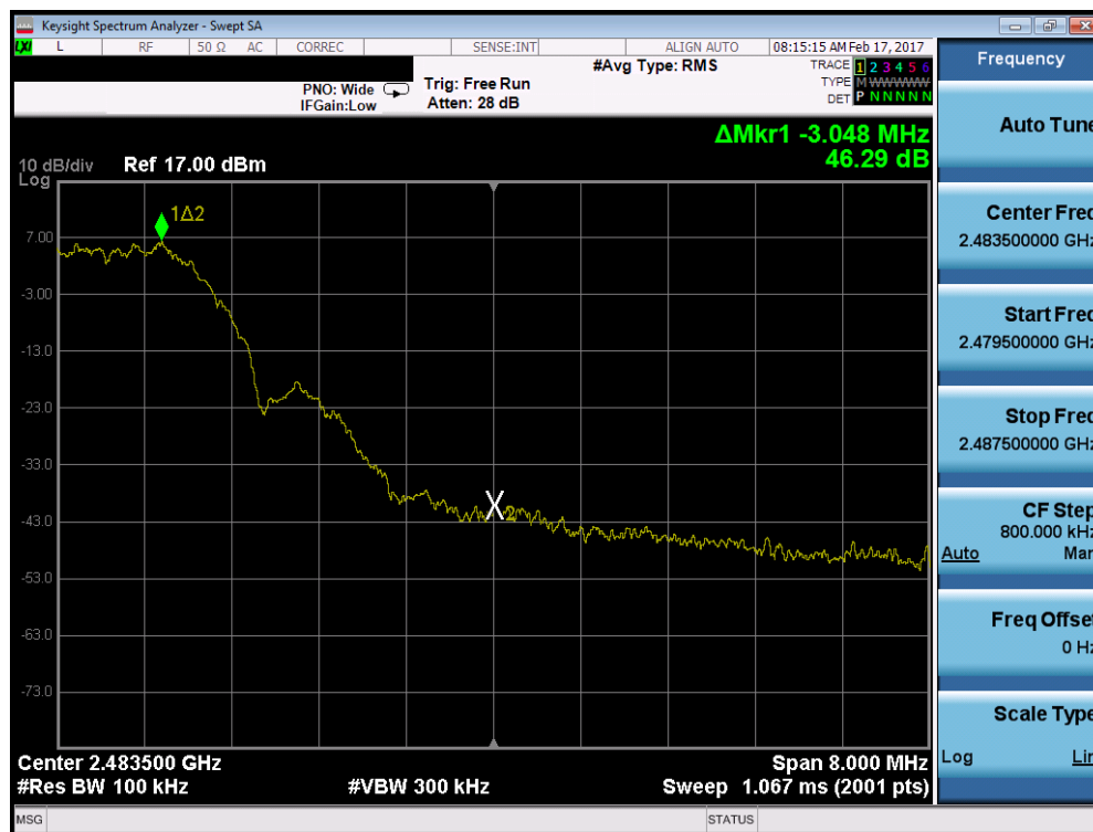
Plot 7-8. Band Edge Plot (ZigBee – Ch. 25)
