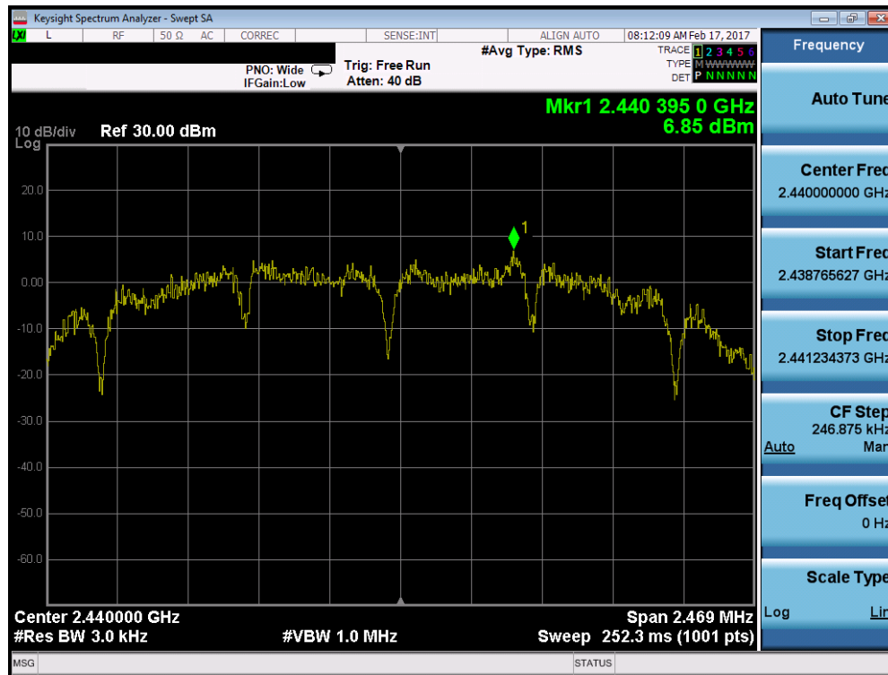
Plot 7-5. Power Spectral Density Plot (ZigBee – Ch. 18)
