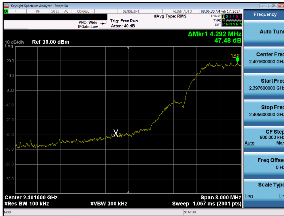
Plot 7-7. Band Edge Plot (ZigBee – Ch. 11)
