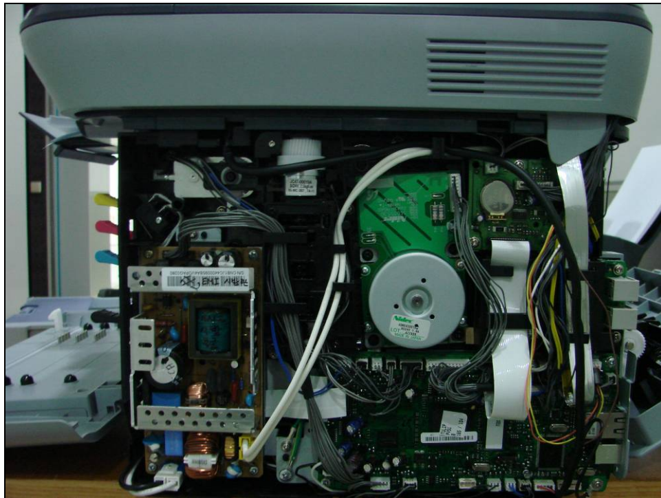
Internal View 1 (Sung-ho SMP board)
