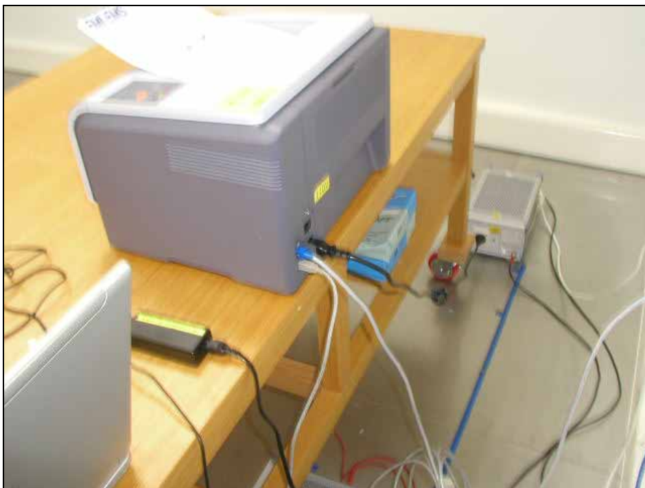
Pic. 2 Conducted Emission (Rear)
