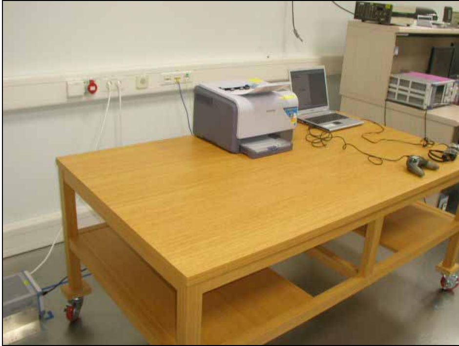
Pic. 1 Conducted Emission (Front)
