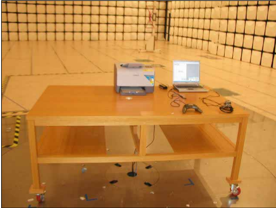
Pic. 3. Radiated Emission (Front)
