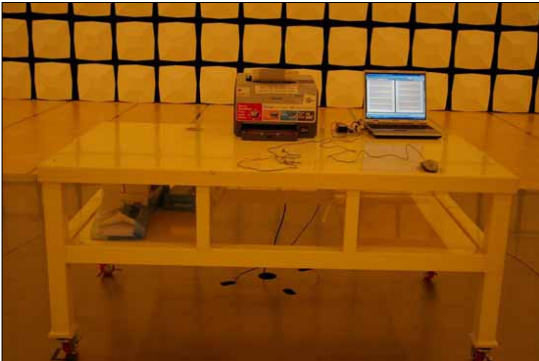
Picture 3. Radiated emission (Front)
