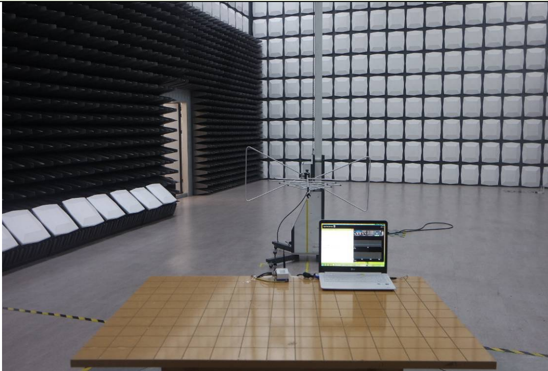
Test Setup for 30 MHz – 1 GHz
