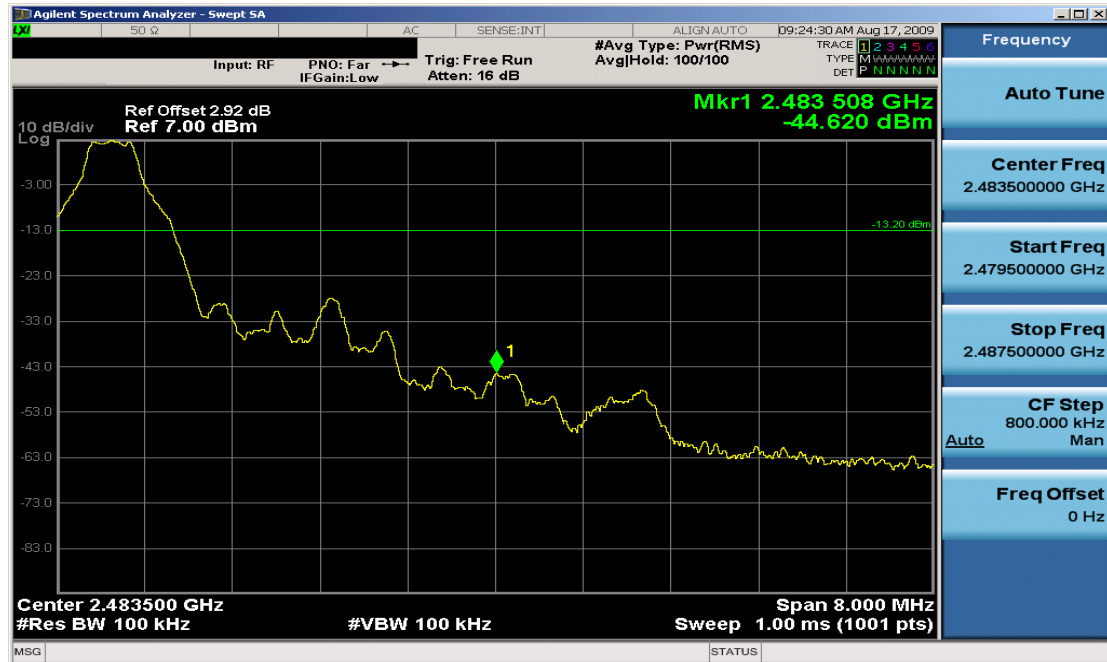
Plot 6-5. Band Edge Plot (Bluetooth – Ch. 78)
