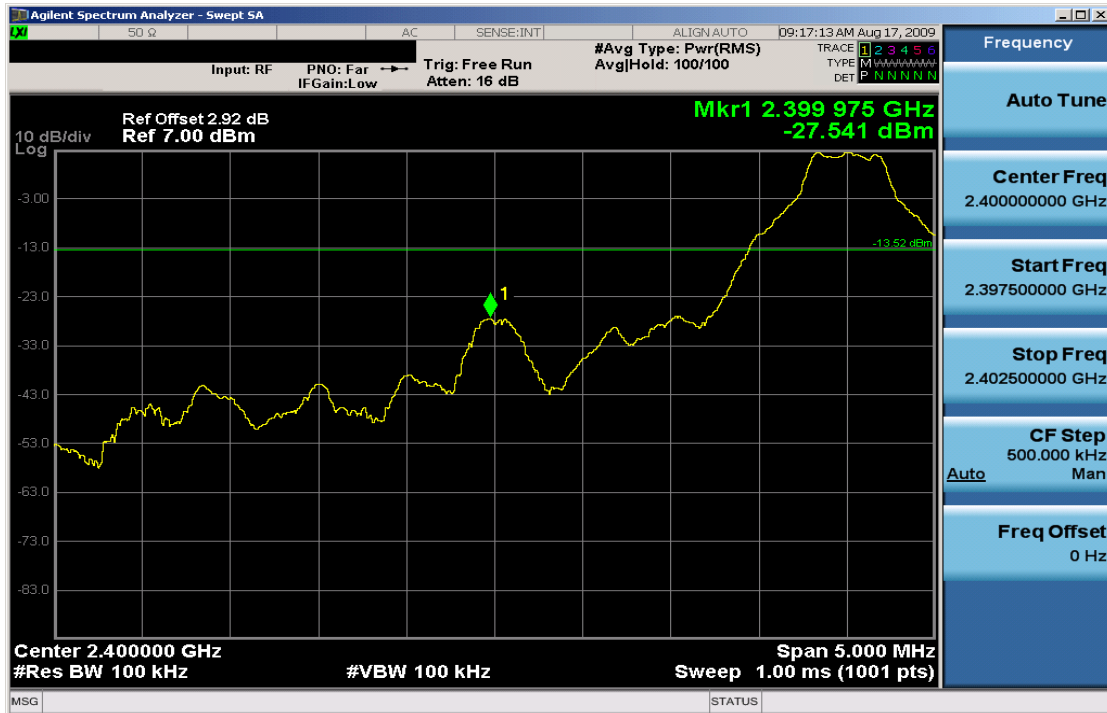
Plot 6-4. Band Edge Plot (Bluetooth – Ch. 0)
