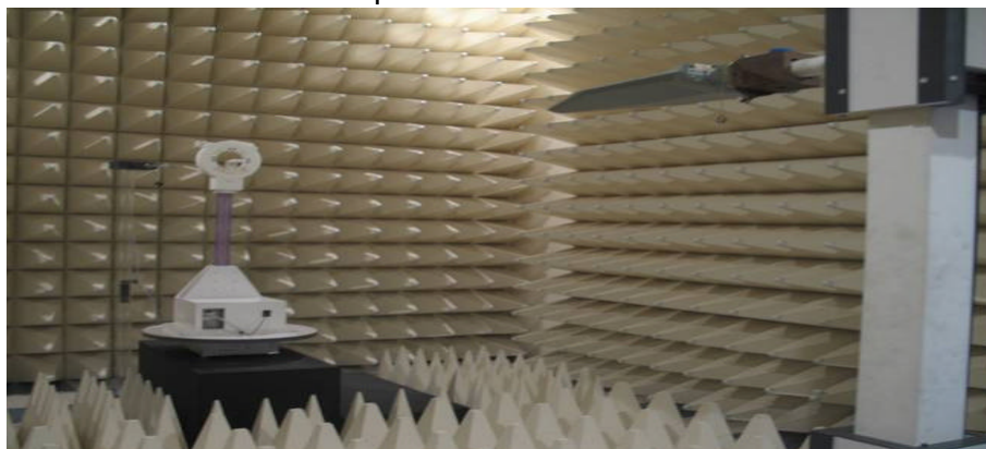
Figure2. Photograph of 3m Fully-Anechoic Chamber
