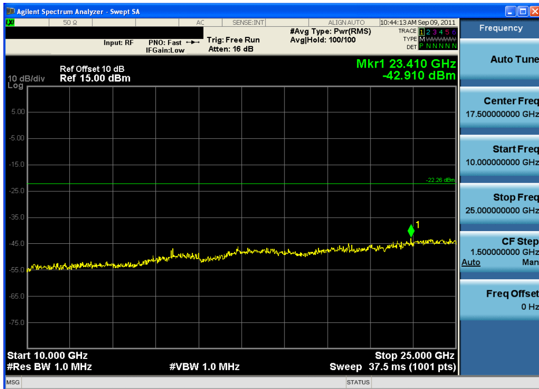
Plot 6-30. Conducted Spurious Plot (802.11b – Ch. 11)
