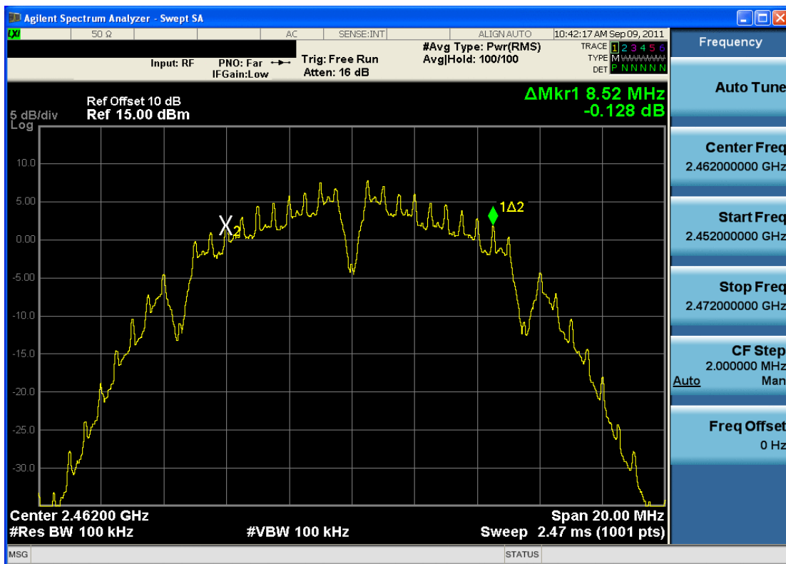
Plot 6-3. 6dB Bandwidth Plot (802.11b – Ch. 11)
