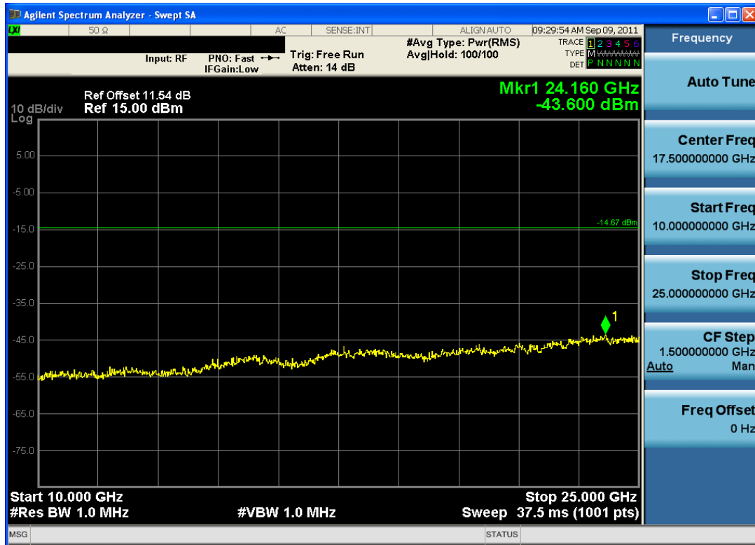
Plot 6-21. Conducted Spurious Plot (Bluetooth, 3Mbps – Ch. 39)
