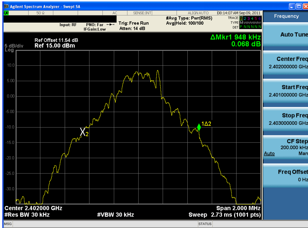
Plot 6-1. 20dB Bandwidth Plot (Bluetooth, 1Mbps – Ch. 0)
