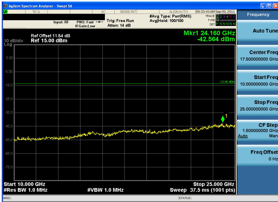
Plot 6-23. Conducted Spurious Plot (Bluetooth, 3Mbps – Ch. 78)
