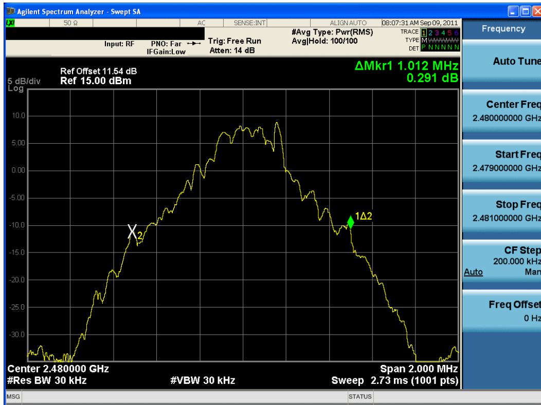
Plot 6-3. 20dB Bandwidth Plot (Bluetooth, 1Mbps – Ch. 78)
