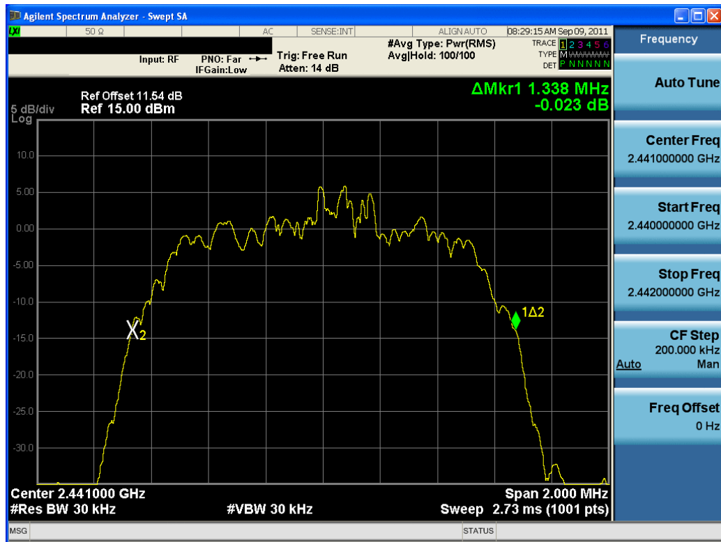
Plot 6-5. 20dB Bandwidth Plot (Bluetooth, 2Mbps – Ch. 39)
