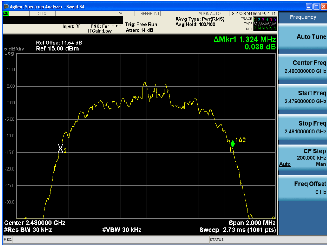
Plot 6-9. 20dB Bandwidth Plot (Bluetooth, 3Mbps – Ch. 78)
