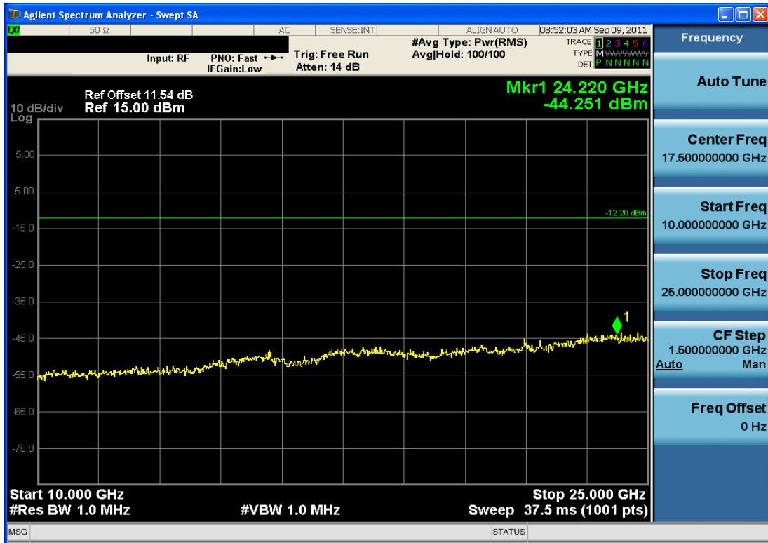
Plot 6-19. Conducted Spurious Plot (Bluetooth, 3Mbps – Ch. 0)
