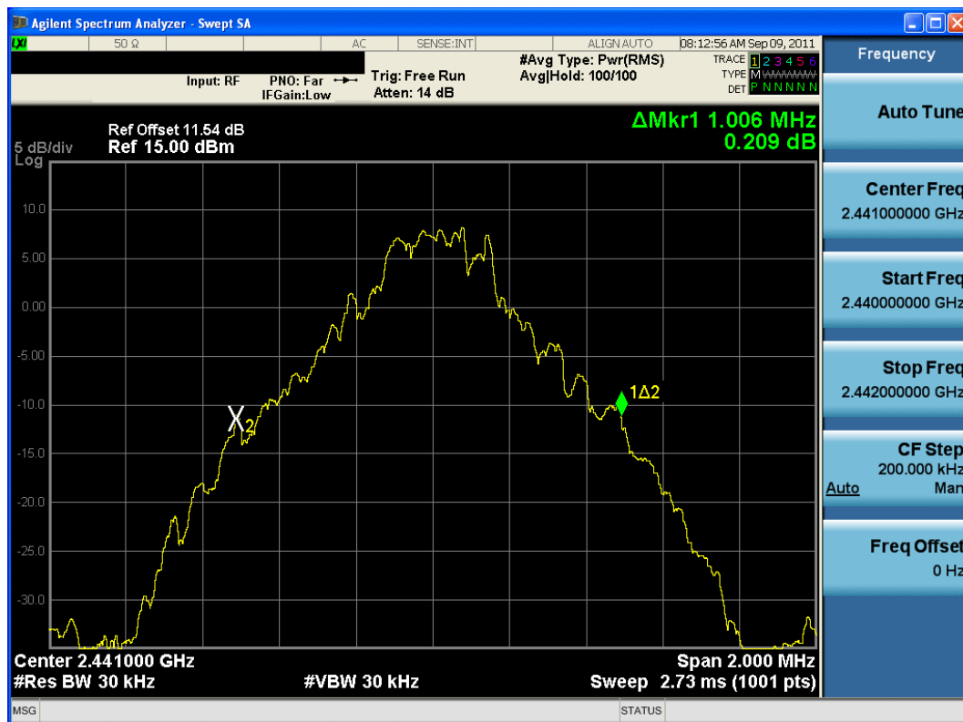
Plot 6-2. 20dB Bandwidth Plot (Bluetooth, 1Mbps – Ch. 39)
