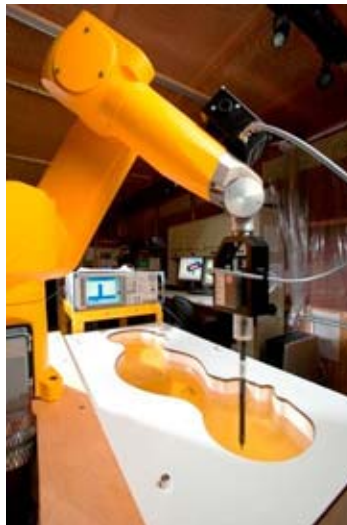
Figure 3-2 DASY4 SAR Measurement System
