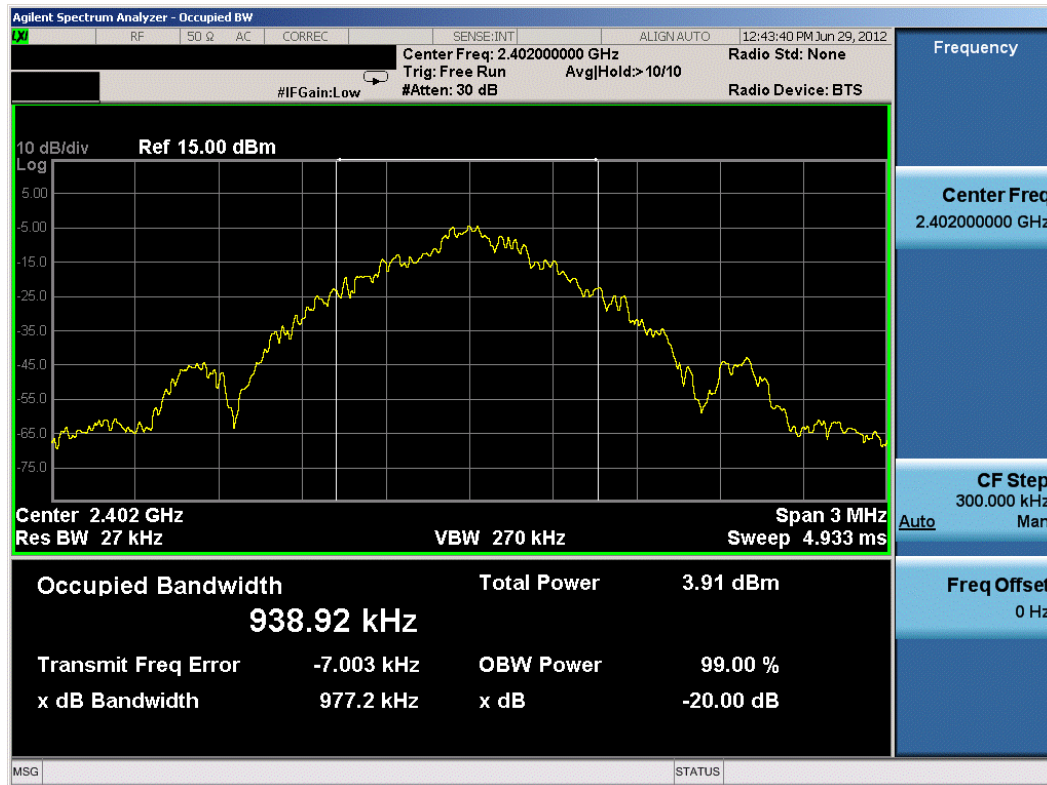
Plot 6-1. 20dB Bandwidth Plot (Bluetooth, 1Mbps – Ch. 0)
