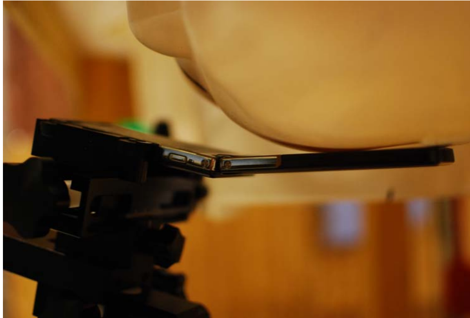
SAR Test Setup Photo 3: Left Touch
