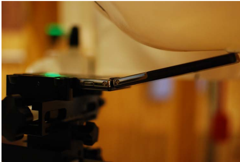
SAR Test Setup Photo 4: Left Tilt
