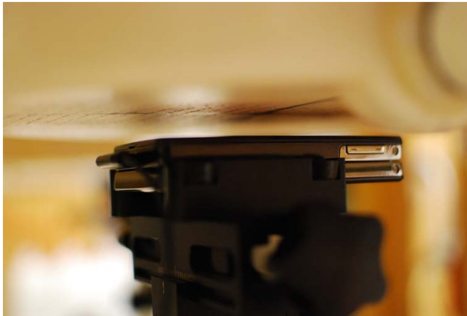
SAR Test Setup Photo 10: Body-Worn at 1.0 cm
