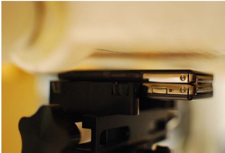
SAR Test Setup Photo 6: Front at 1.0 cm
