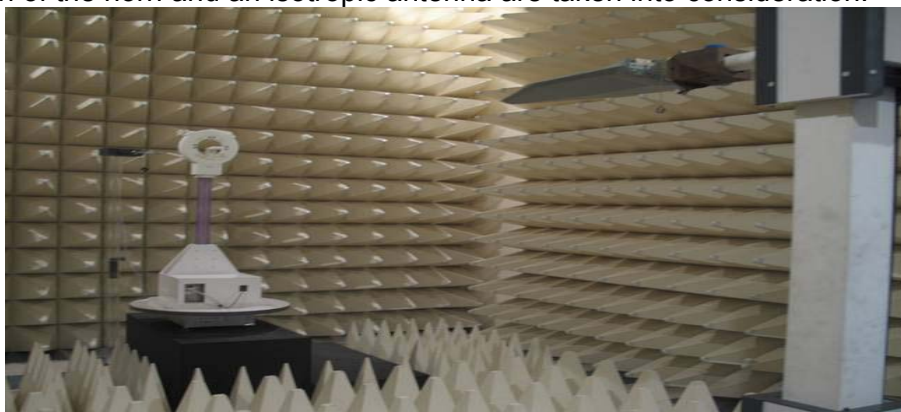
Figure2. Photograph of 3m Fully-Anechoic Chamber
