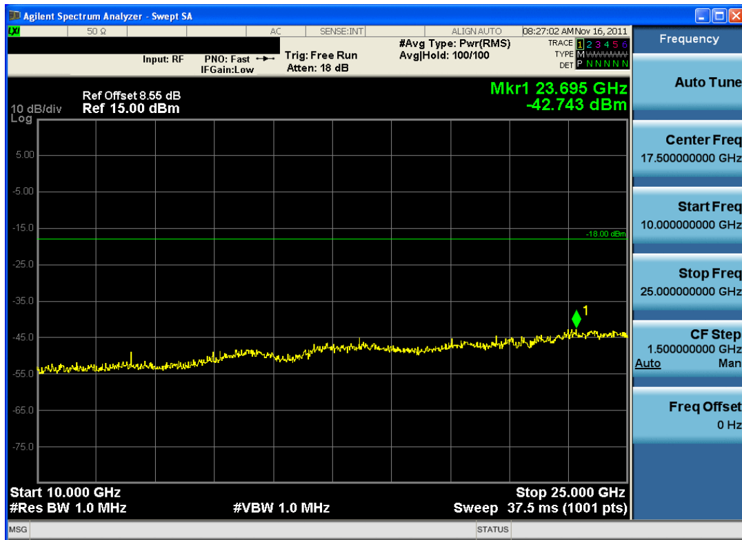
Plot 6-21. Conducted Spurious Plot (Bluetooth, 1Mbps – Ch. 78)
