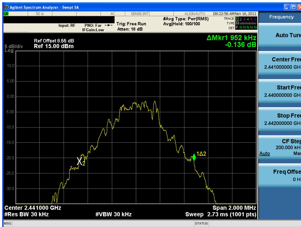
Plot 6-2. 20dB Bandwidth Plot (Bluetooth, 1Mbps – Ch. 39)
