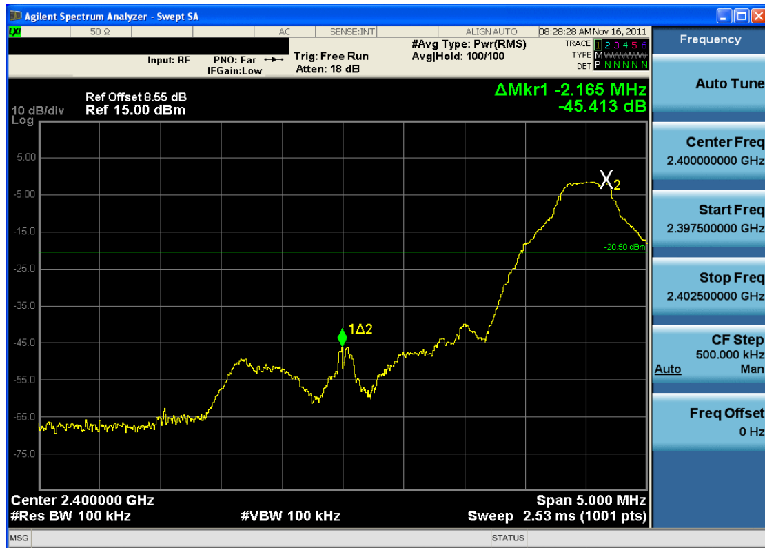
Plot 6-10. Band Edge Plot (Bluetooth, 1Mbps – Ch. 0)
