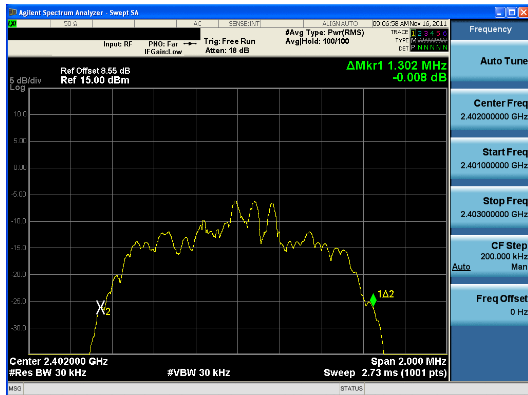
Plot 6-4. 20dB Bandwidth Plot (Bluetooth, 2Mbps – Ch. 0)
