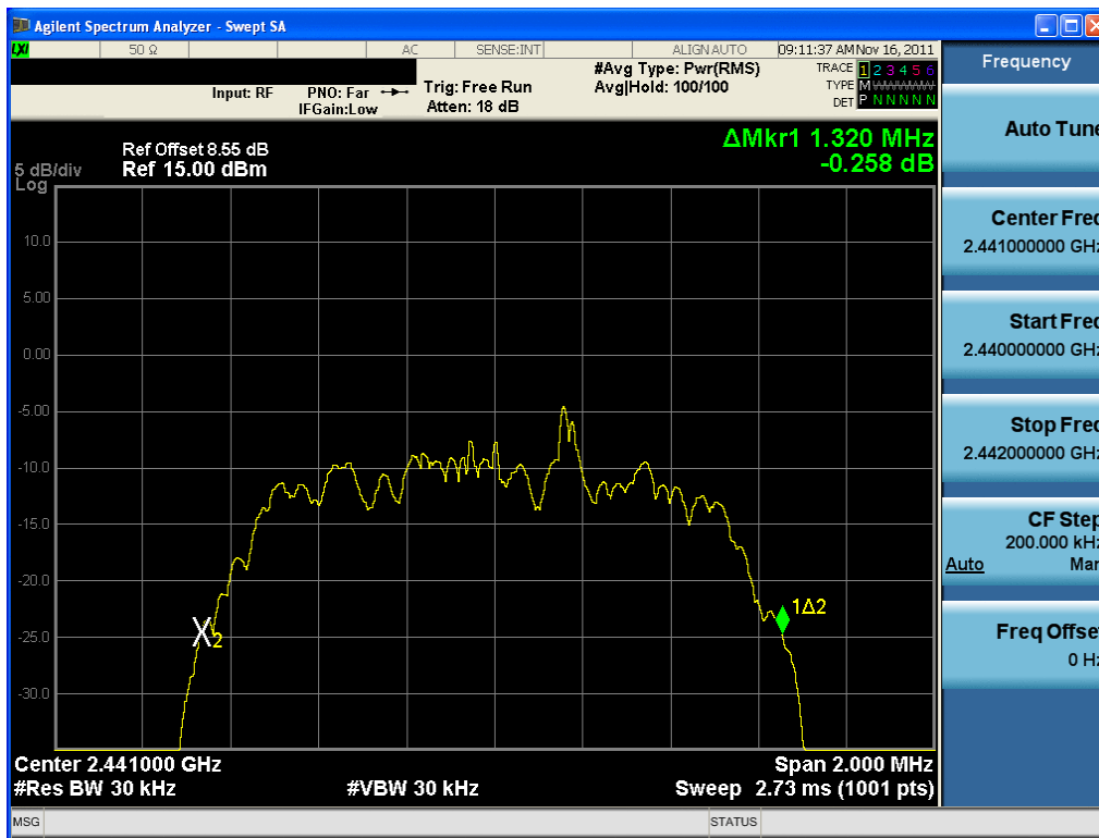
Plot 6-5. 20dB Bandwidth Plot (Bluetooth, 2Mbps – Ch. 39)
