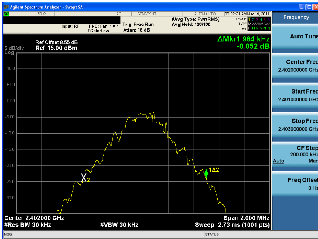
Plot 6-1. 20dB Bandwidth Plot (Bluetooth, 1Mbps – Ch. 0)
