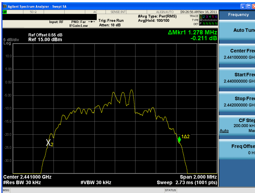
Plot 6-8. 20dB Bandwidth Plot (Bluetooth, 3Mbps – Ch. 39)
