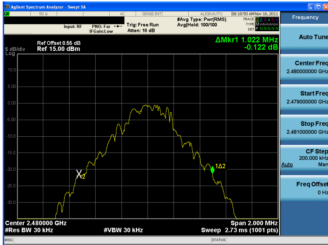
Plot 6-3. 20dB Bandwidth Plot (Bluetooth, 1Mbps – Ch. 78)
