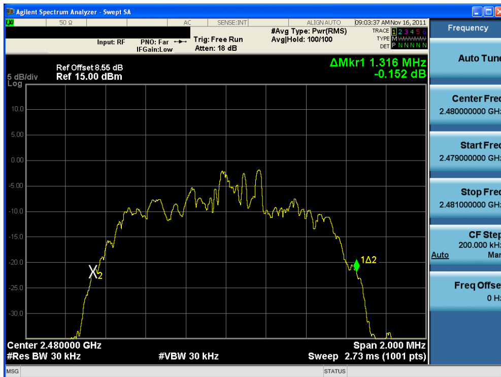
Plot 6-6. 20dB Bandwidth Plot (Bluetooth, 2Mbps – Ch. 78)
