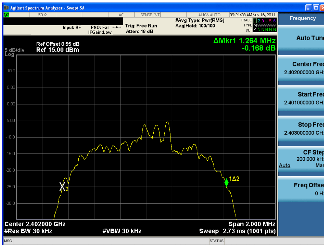
Plot 6-7. 20dB Bandwidth Plot (Bluetooth, 3Mbps – Ch. 0)
