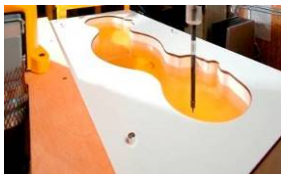
Figure 6-2 SAM Phantom with Simulating Tissue
