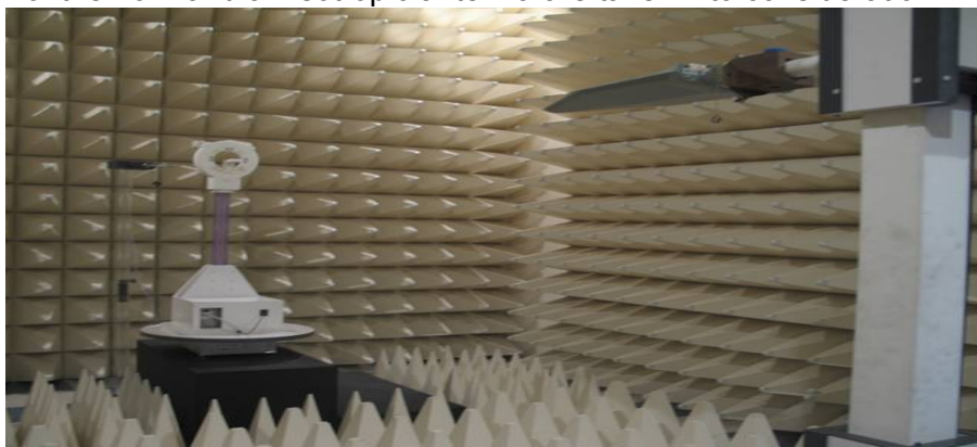
Figure2. Photograph of 3m Fully-Anechoic Chamber
