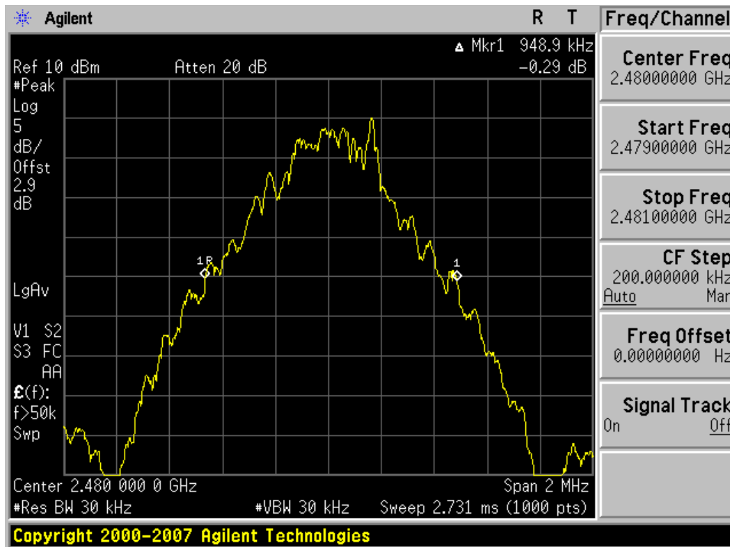
Plot 6-3. 20dB Bandwidth Plot (Bluetooth, 1Mbps – Ch. 78)
