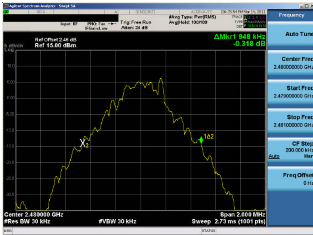
Plot 6-3. 20dB Bandwidth Plot (Bluetooth, 1Mbps – Ch. 78)
