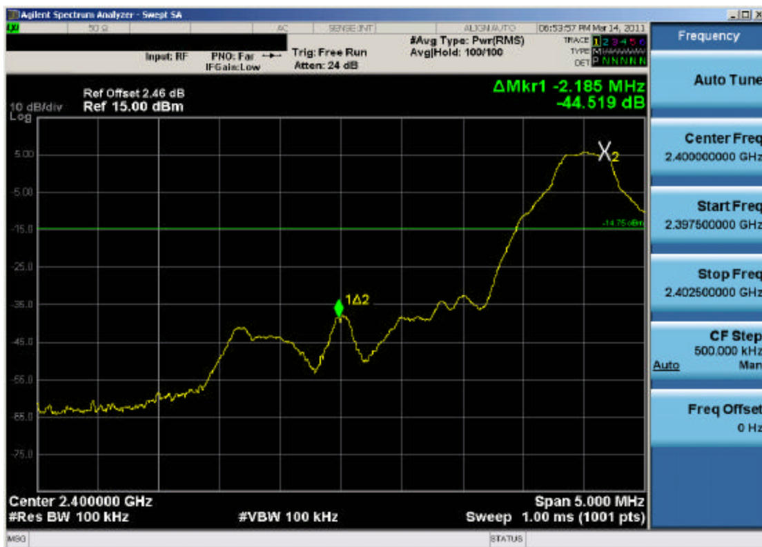
Plot 6-10. Band Edge Plot (Bluetooth, 1Mbps – Ch. 0)
