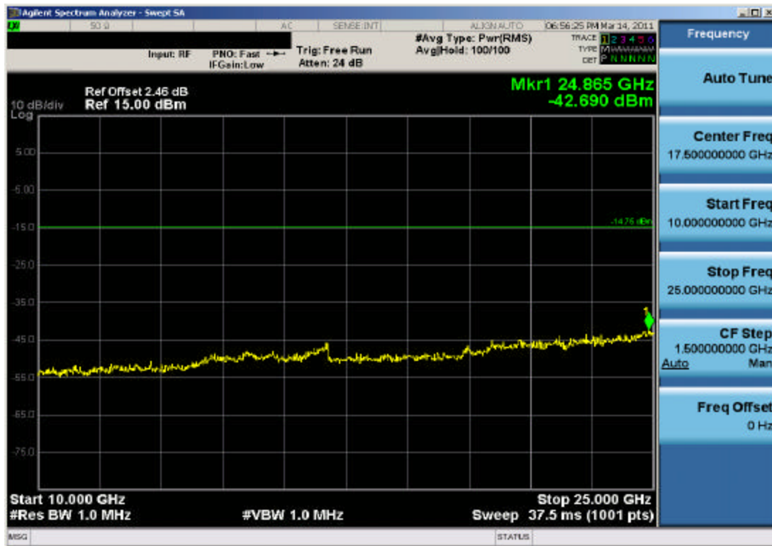
Plot 6-19. Conducted Spurious Plot (Bluetooth, 1Mbps – Ch. 0)
