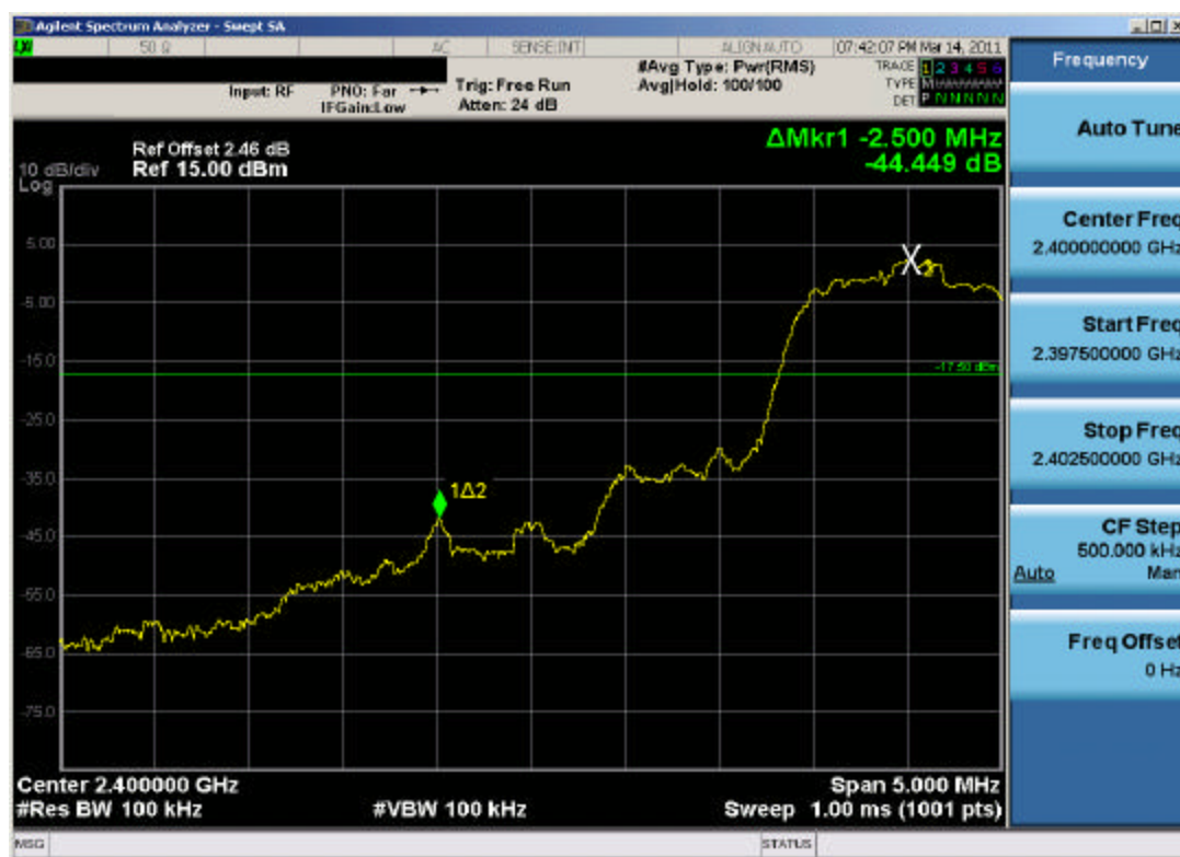
Plot 6-12. Band Edge Plot (Bluetooth, 3Mbps – Ch. 0)
