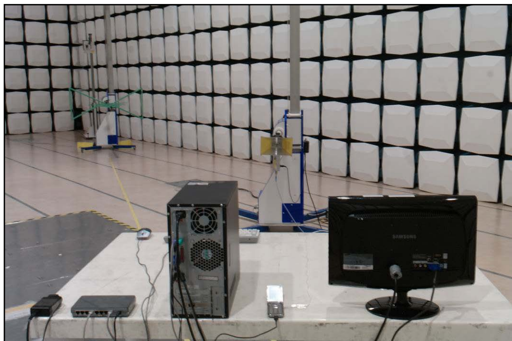
[ Radiated Disturbance for Above 1 GHz – Rear ]
