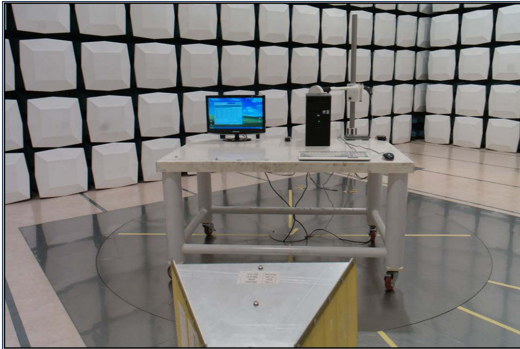
[ Radiated Disturbance for Above 1 GHz – Front ]
