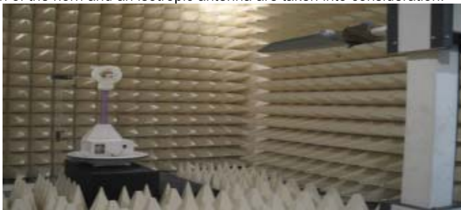
Figure2. Photograph of 3m Fully-Anechoic Chamber
