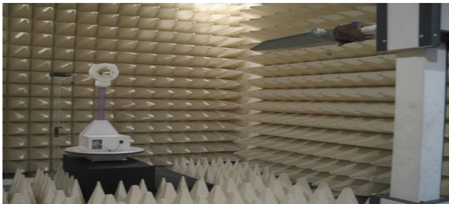
Figure2. Photograph of 3m Fully-Anechoic Chamber
