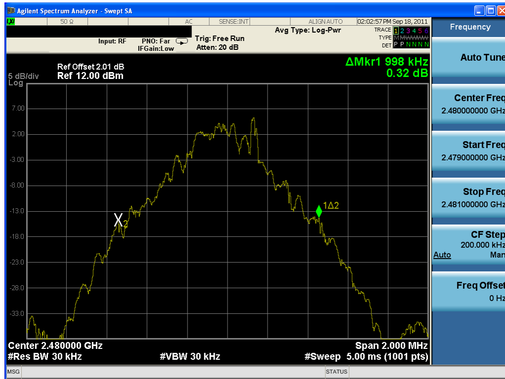
Plot 6-3. 20dB Bandwidth Plot (Bluetooth, 1Mbps – Ch. 78)
