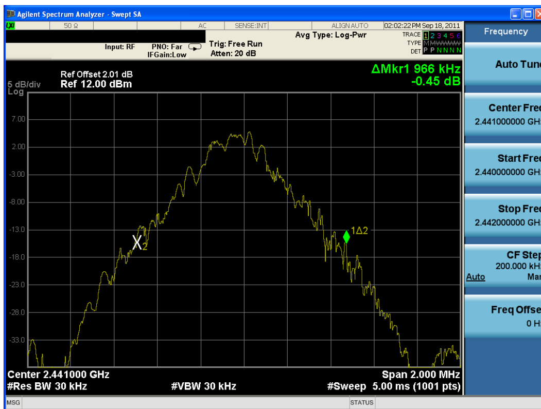
Plot 6-2. 20dB Bandwidth Plot (Bluetooth, 1Mbps – Ch. 39)
