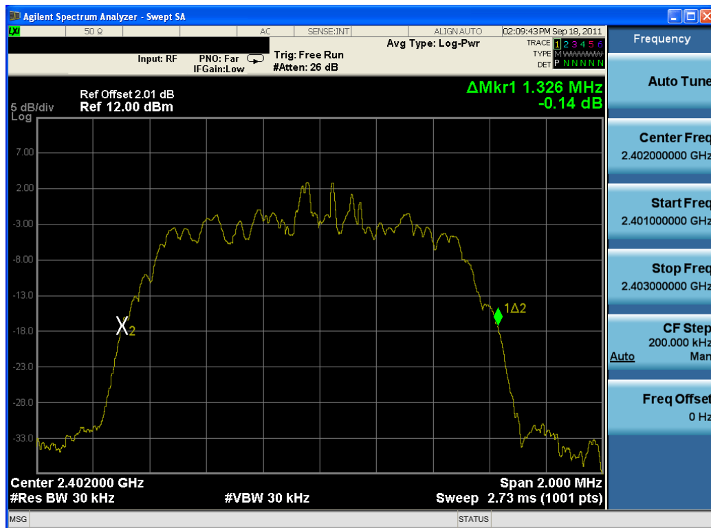
Plot 6-4. 20dB Bandwidth Plot (Bluetooth, 2Mbps – Ch. 0)
