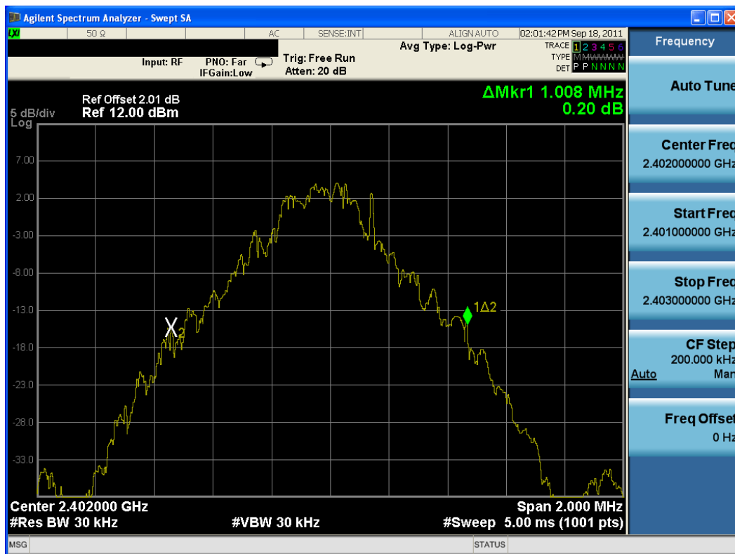
Plot 6-1. 20dB Bandwidth Plot (Bluetooth, 1Mbps – Ch. 0)
