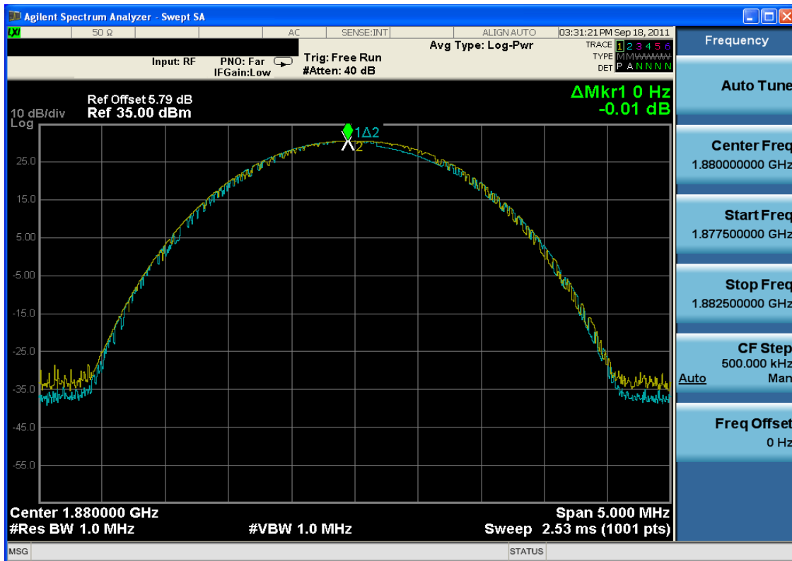
Plot 7-22. Peak-Average Ratio Plot (EDGE1900 Mode – Ch. 661)
