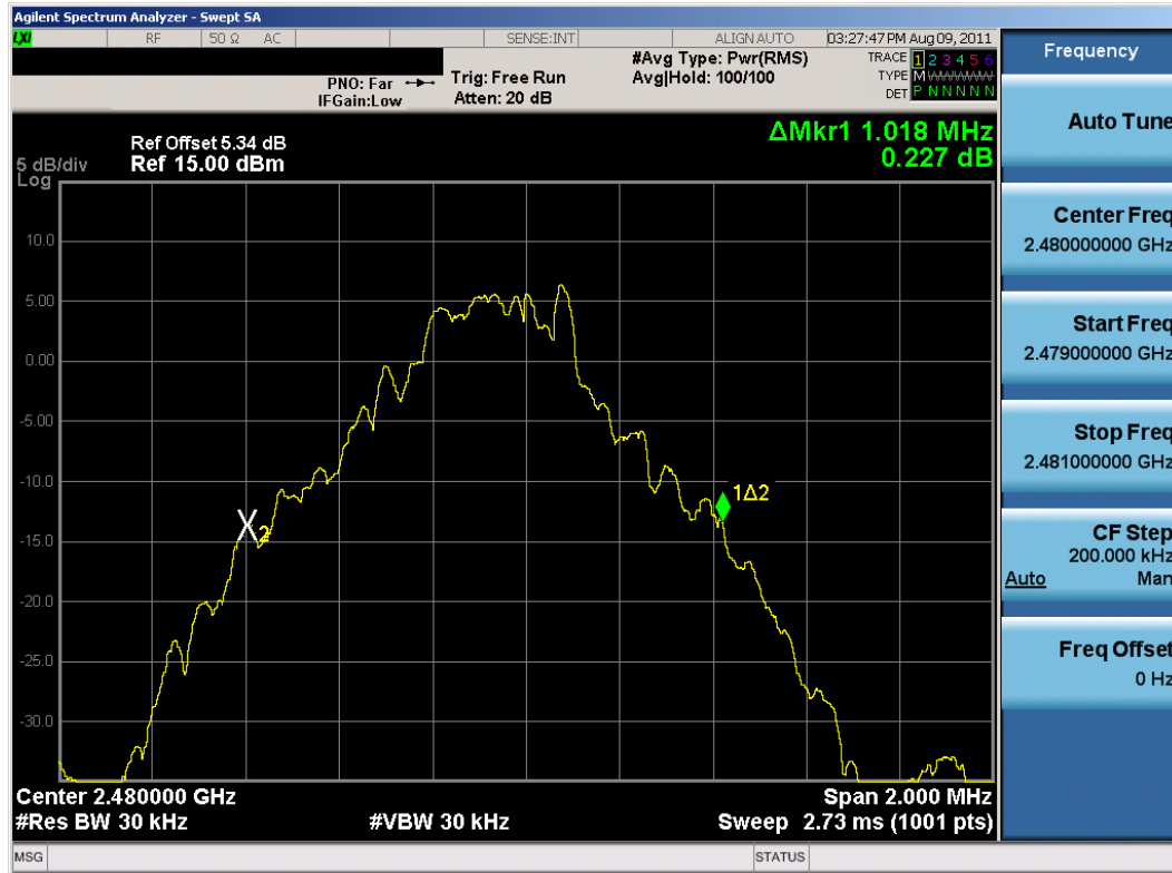
Plot 6-3. 20dB Bandwidth Plot (Bluetooth, 1Mbps – Ch. 78)
