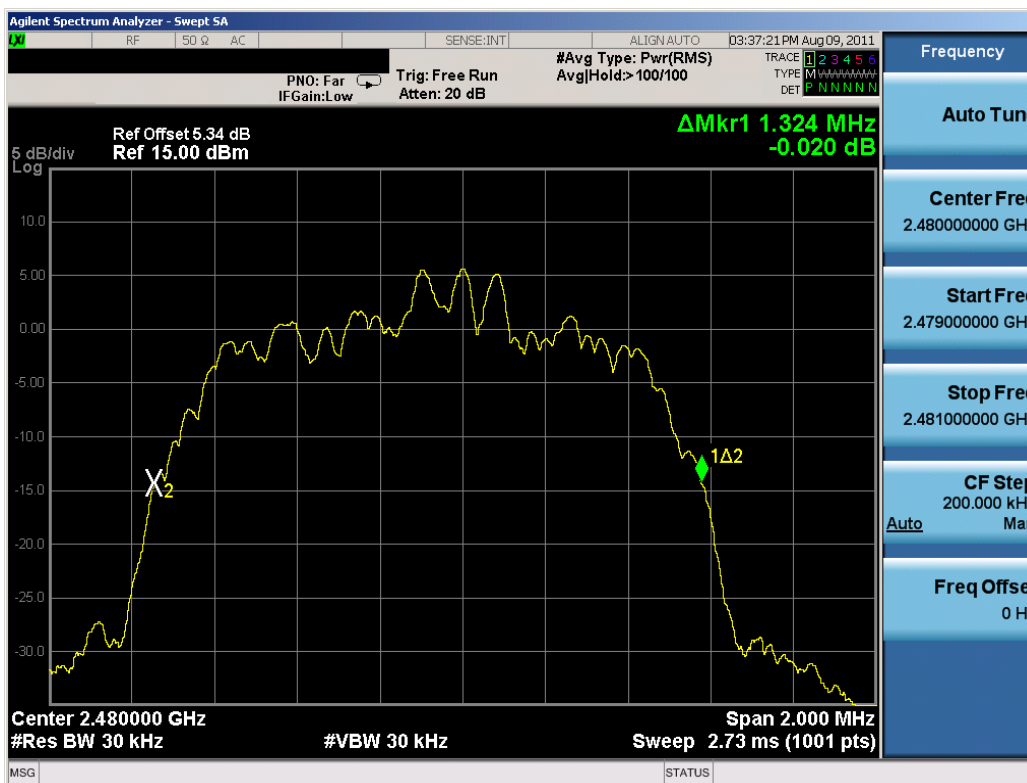
Plot 6-6. 20dB Bandwidth Plot (Bluetooth, 2Mbps - Ch. 78)
