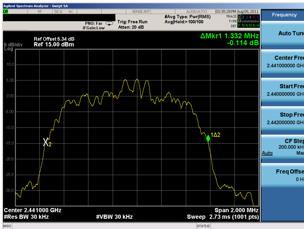
Plot 6-5. 20dB Bandwidth Plot (Bluetooth, 2Mbps - Ch. 39)
