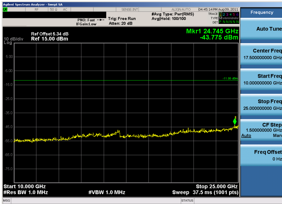
Plot 6-21. Conducted Spurious Plot (Bluetooth, 2Mbps – Ch. 78)
