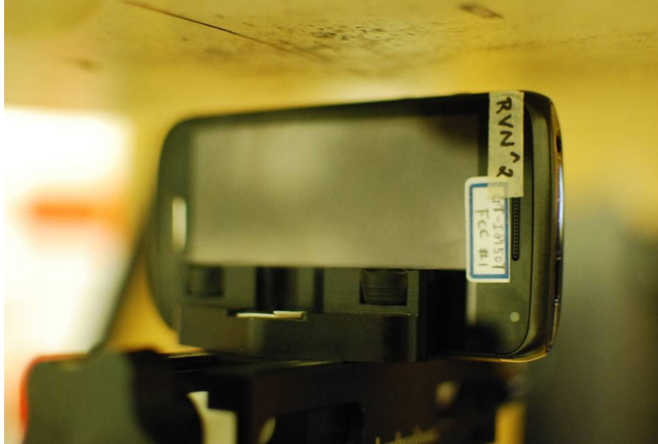
SAR Test Setup Photo 9 – Left at 1.0 cm
