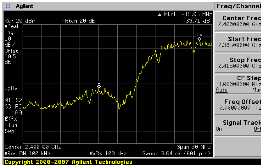
Plot 6-13. Band Edge Plot (802.11b – Ch. 1)
