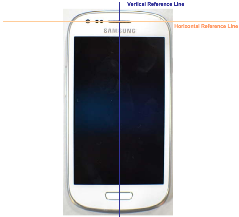
SAR Test Setup Photo 11 – DUT Vertical and Horizontal Reference Lines
