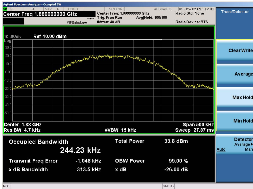
Plot 7-18. Occupied Bandwidth Plot (PCS GSM Mode – Ch. 661)
