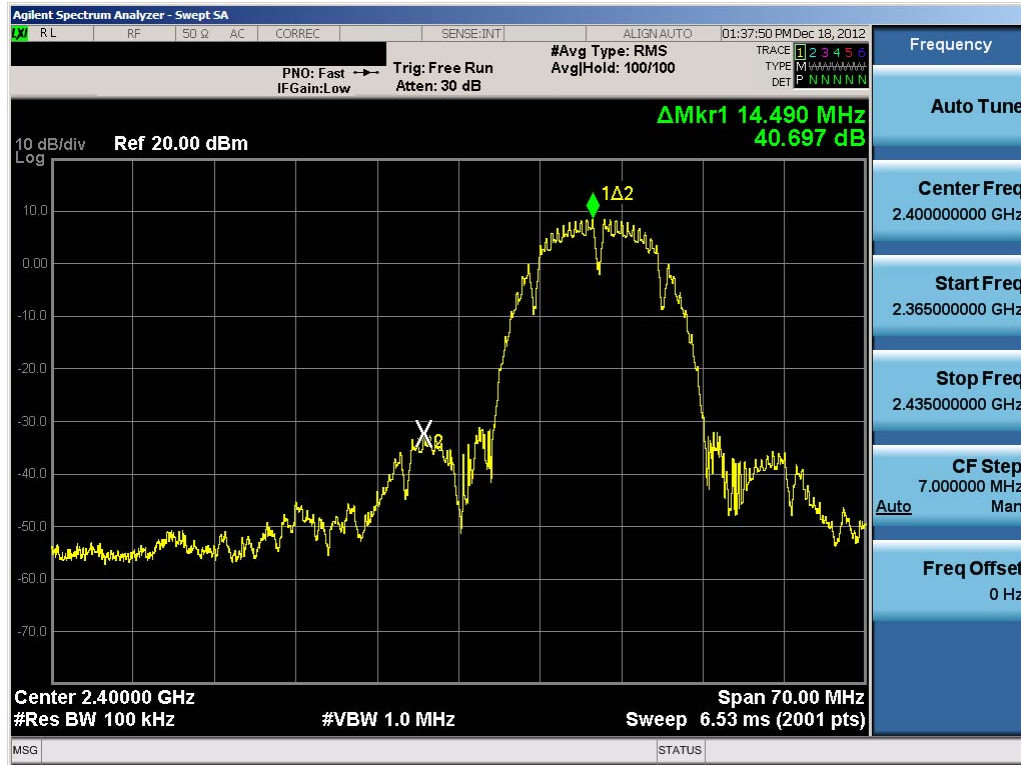
Plot 6-19. Band Edge Plot (802.11b – Ch. 1)
