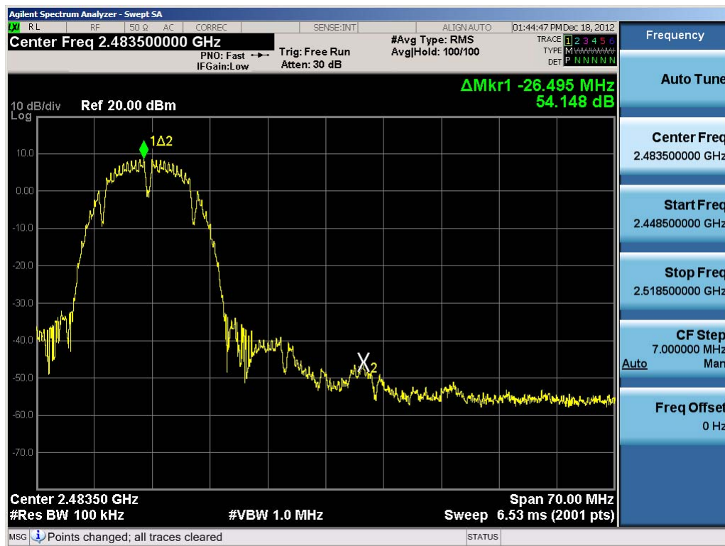
Plot 6-20. Band Edge Plot (802.11b – Ch. 11)
