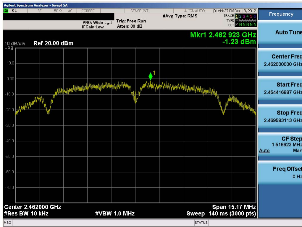
Plot 6-12. Power Spectral Density Plot (802.11b – Ch. 11)
