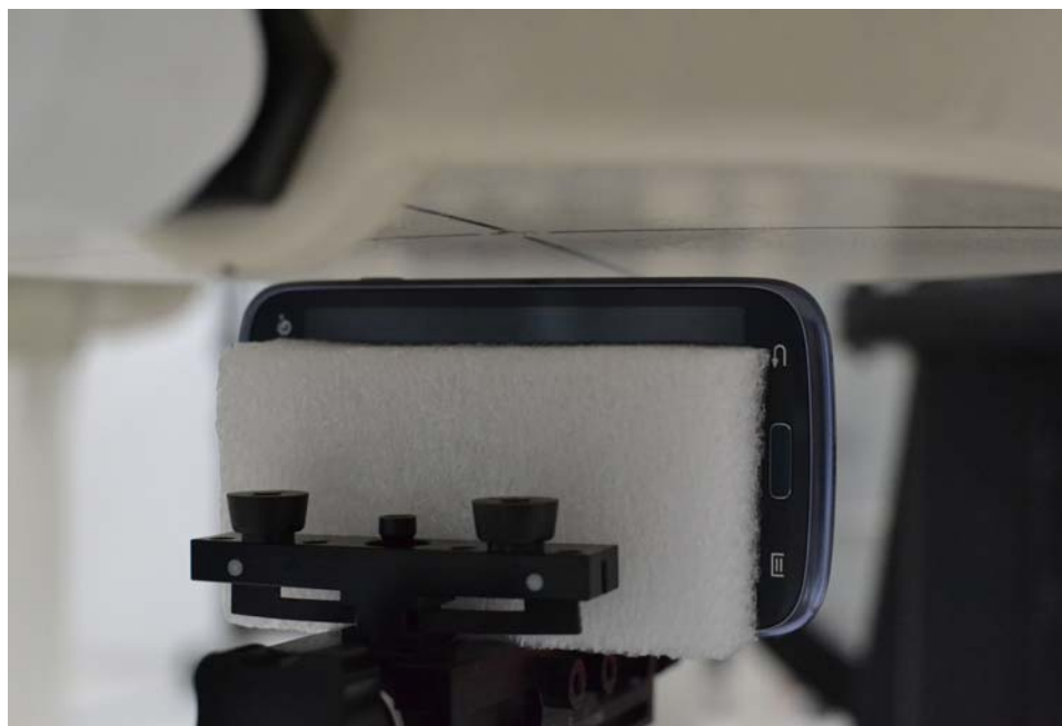
SAR Test Setup Photo 9 - Right Side at 1.0 cm
