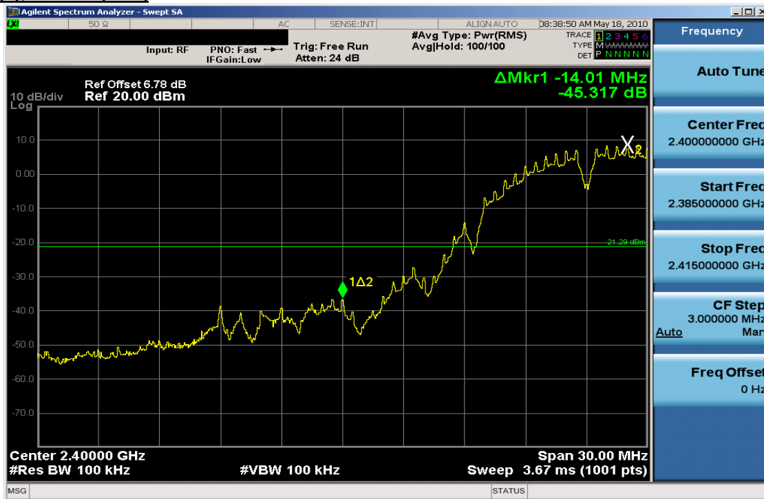
Plot 6-19. Band Edge Plot (802.11b – Ch. 1)
