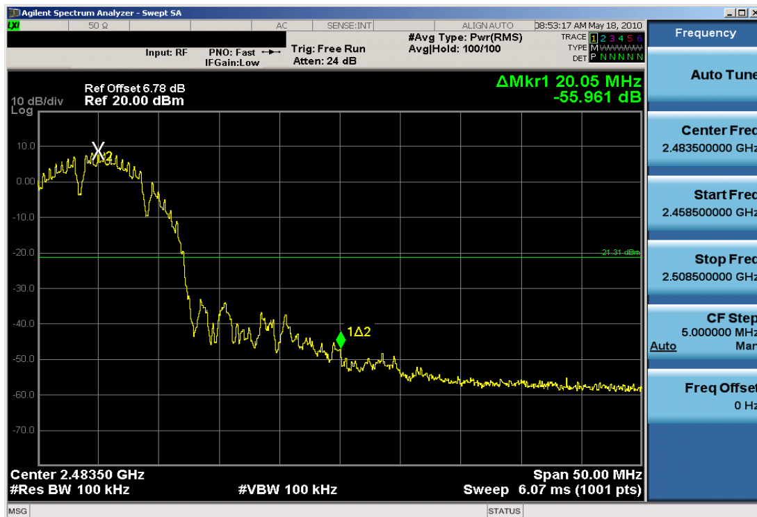
Plot 6-20. Band Edge Plot (802.11b – Ch. 11)
