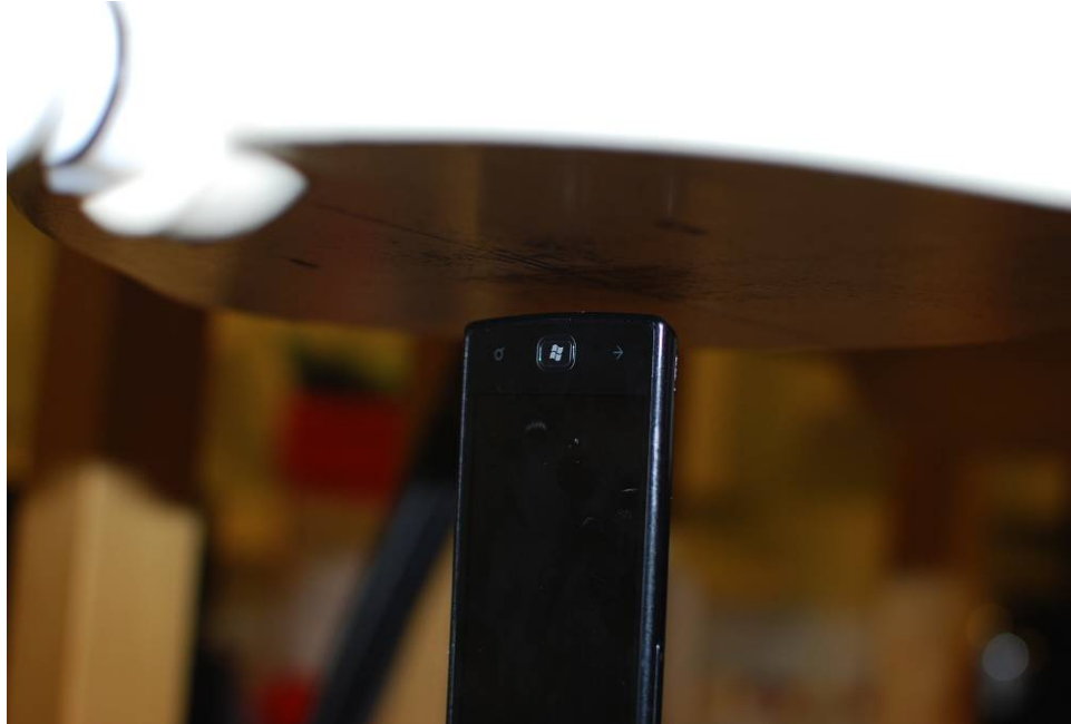
SAR Test Setup Photo 8 – Bottom at 1.0 cm
