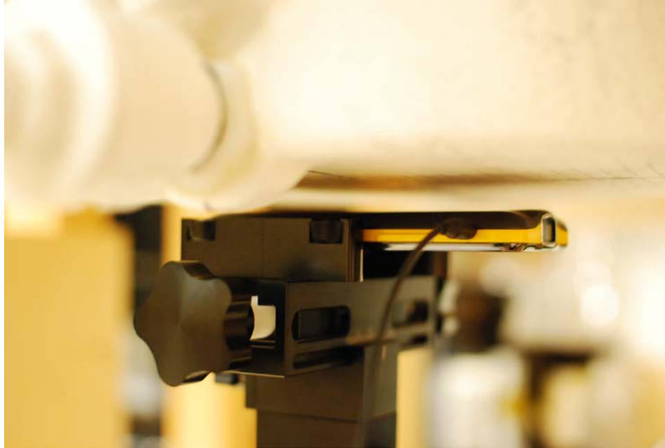
SAR Test Setup Photo 11 – Body-worn at 1.0 cm
