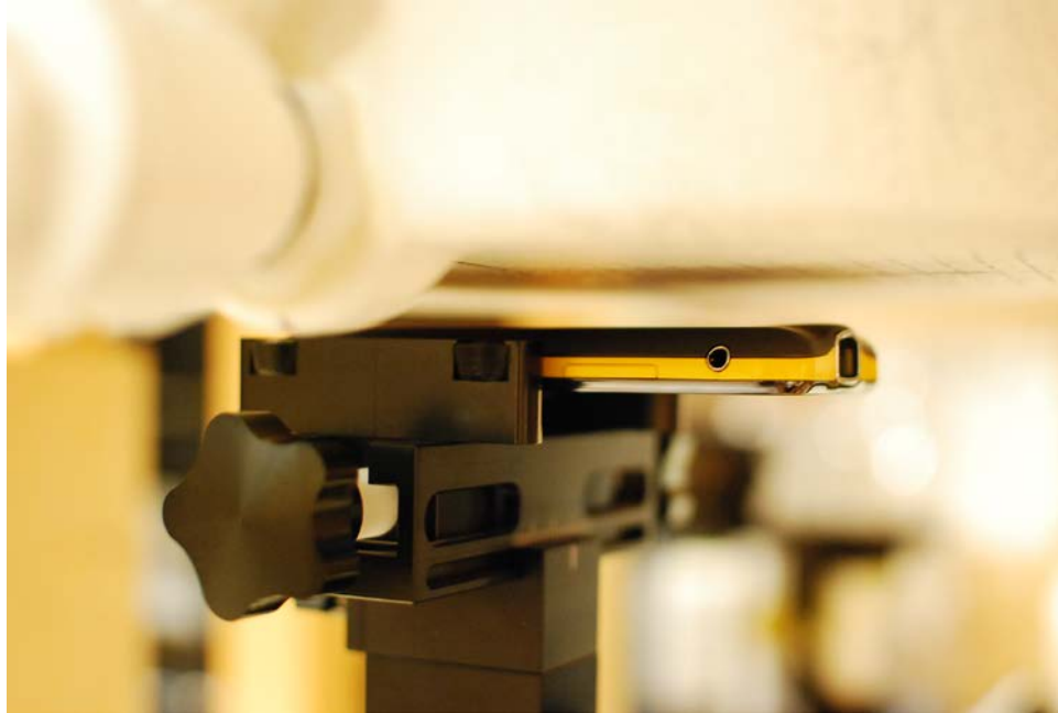
SAR Test Setup Photo 5 – Back at 1.0 cm
